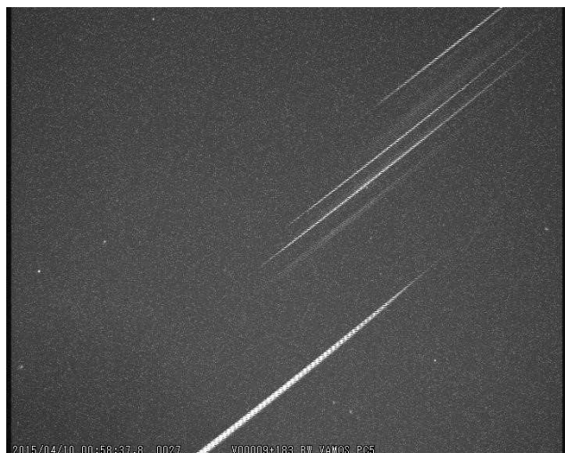
Figure 2 – Meteor and spectrum captured by B. Ward, Kilwinning, Scotland. Camera: Watec 902H2 Ultimate. Lens: 12 mm f/0.8 , grating: 600 lines/mm (fused silica substrate).
